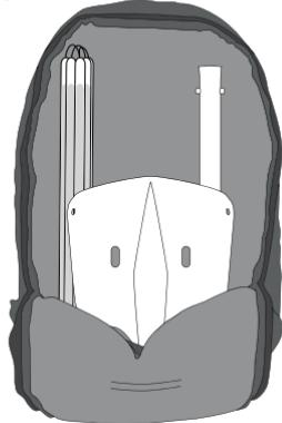
Placing the blade in this direction reduces wear on the bottom of the pack from the blade edge, and removes a pressure point on the inflation system and pack contents.
